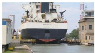
Heading west we came to the Welland Canal, built to allow large vessels to bypass the Niagara falls and sail via a series of 8 locks between Lake Ontario and Lake Erie and onto Detroit. The ships are made the maximum size possible, allowing only a few inches between the sides of the ship and the lock. It is very impressive. What is not immediately evident is that although Niagara falls look amazing, much
